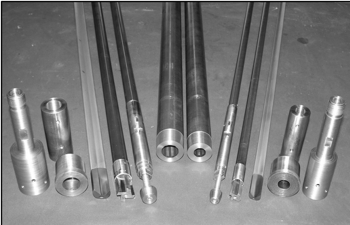
Tools of the trade: 8-bore tooling on the left, 58 caliber tooling on the right. In the center lie two completed barrel blanks, one in each caliber.
